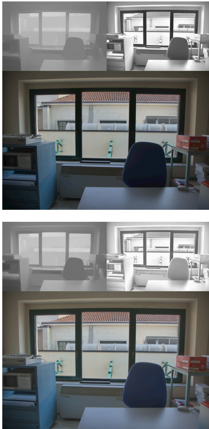
Figure 3.11: Results obtained with the proposed Retinex-like method, using \alpha = 100 (top) and \alpha = 20 (bottom) in the variational filter for the extraction of the illumination component. The estimated illumination and reflectance are shown together with the processed output. The illumination is mapped with the proposed modified logarithmic curve.
