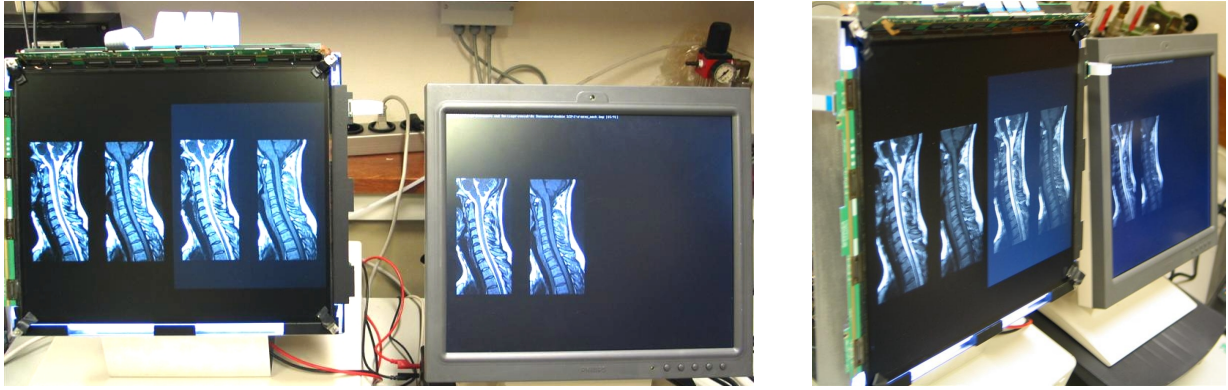
Figure 6.3: Picture of the prototype. Clearly visible is the very good black level in the left part of the left display (the dual layer LCD prototype). The right side of the prototype screen shows the image as it would look on a normal greyscale LCD monitor, which is placed to the right of the prototype for comparison. The right photo shows that also the viewing angle is greatly improved.
