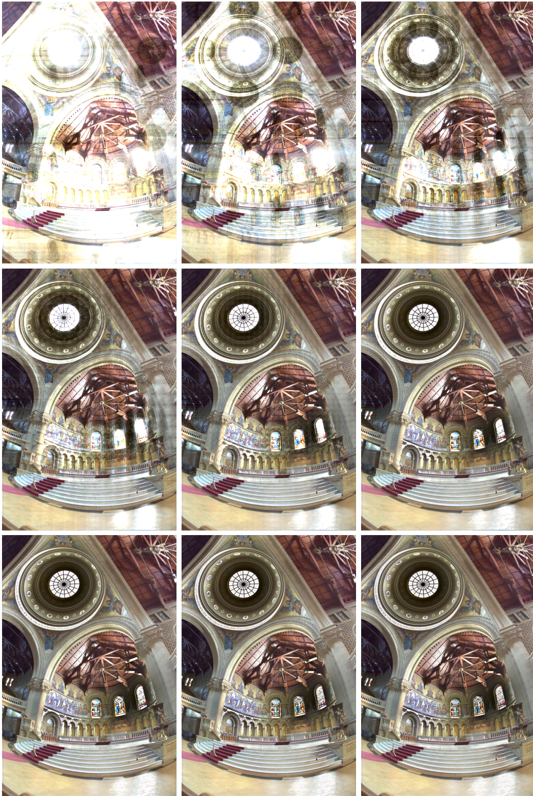
Figure 3.7: Intermediate results of the modified Frackle-McCann Retinex algorithm. The 768 \times 512 image was processed with 4 revolutions per level and an initial displacement of 256 pixels. The 9 images were visualized after each group of 4 revolutions, i.e. with a displacement of 256, 128, 64, 32, 16, 8, 4, 2 and 1 pixels.
