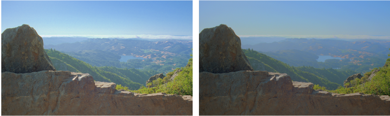
Figure 3.2: Nonlinear mapping on luminance only, with the luminance computed as maximum (left) and weighted average (right) of the RGB channels.
