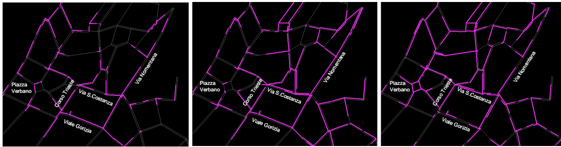
Figure 18. Queue movement across the network as computed by Dynasmart in three different consecutive time instants (from left to right).
