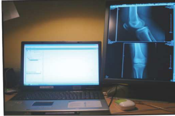
figure 3 – actual implemented home tele-radiology workstation
