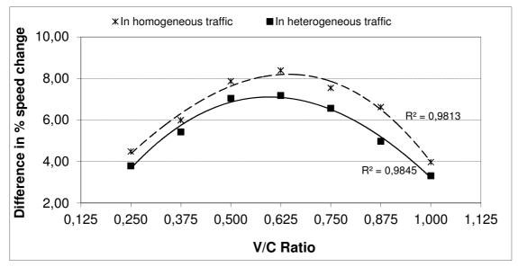
Figure 14: Comparison of difference in speed change between cars and buses under homogeneous and heterogeneous traffic condition.
