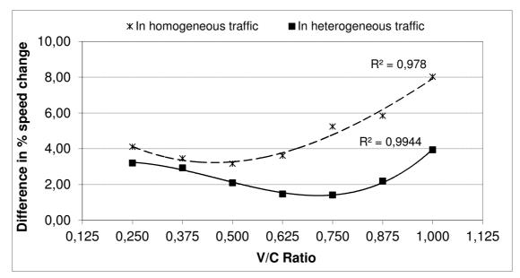
Figure 13: Comparison of difference in speed change between cars and buses under homogeneous and heterogeneous traffic condition.
