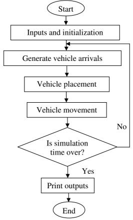
Figure 2: Flow diagram of the simulation model.
