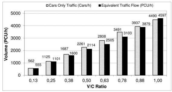
Figure 15: Comparison of heterogeneous traffic and cars-only traffic flows.
