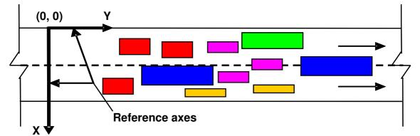
Figure 1: Reference axes for representing vehicle positions.
