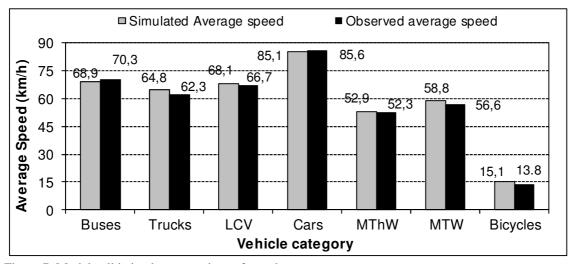
Figure 7: Model validation by comparison of speeds. Note: L.C.V. - Light Commercial Vehicles; M.Th.W. - Motorised Three-Wheelers; M.T.W. - Motorised Two-Wheelers.
