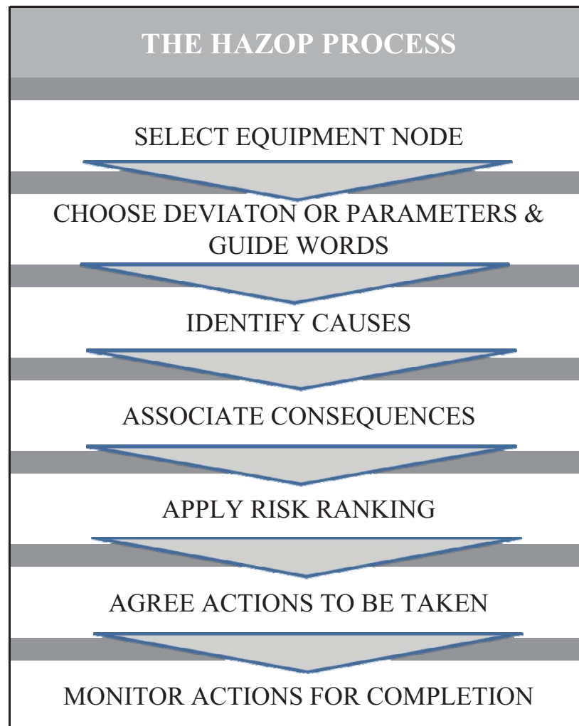
Figure 3.14: A block flow diagram of the HAZOP process
