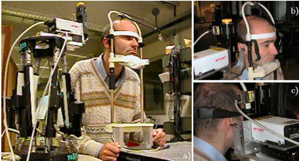
Figure 6.7: Otoscan3D in-vivo measurements: a) patient is immobilized with the help of a frame; b) positioning of the probe and tragus opening; c) scan of the EAC.
