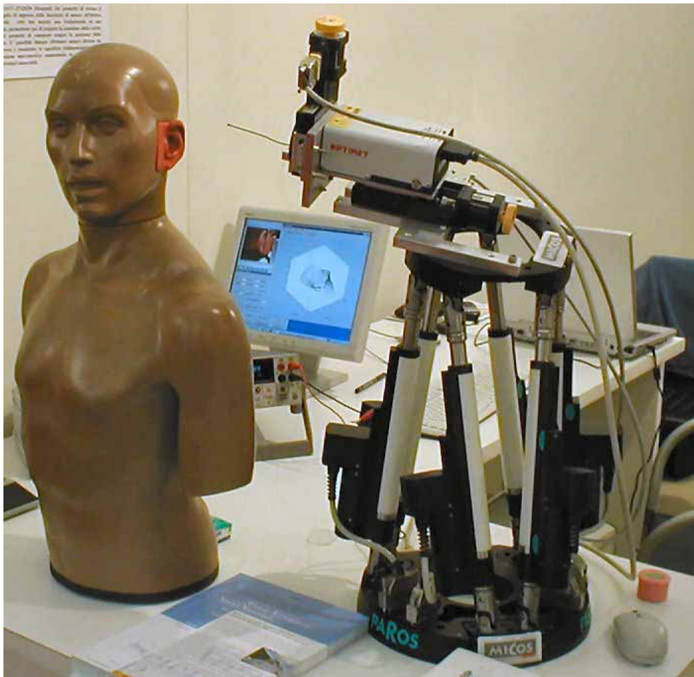
Figure 5.1: prototype Otoscan3D: 3D laser scanner based on surface silicon micromachining techniques for shape and size reconstruction of the human ear canal.
