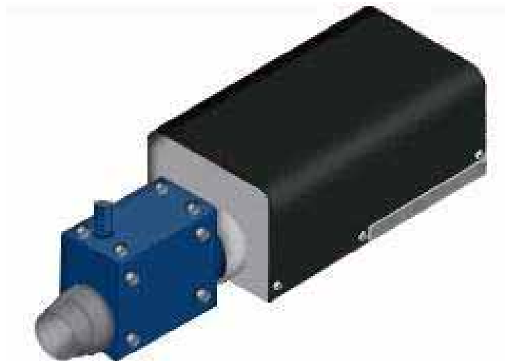
Figure 7.1: Otoscan3D improvement: a video camera is inserted between the ConoProbe and the objective lens
