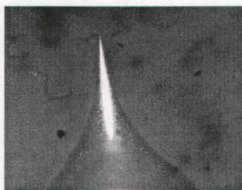
Figure 1.6: A typical STM tip obtained by etching of a 0.38 mm wide W wire.
