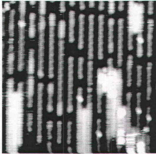
Figure 4.13: Second reaction step proceeding from the segment ends all over the surface. Reacted parts appear brighter. Size: 150 \times 150 \text{ \AA}^2 . ( I=1.00 \text{ nA} , V_B=+0.60 \text{ V} ).
