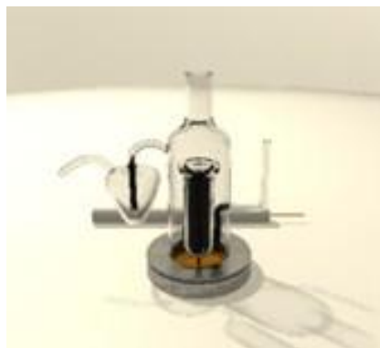
Figure 2-8. Three-electrode half-cell used in in-situ Fourier Transform Infrared (FTIR) spectroscopy.
