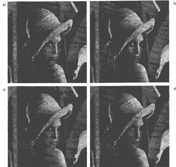
Figure 3.12: Blocking artifacts removing Filter: a) original image, b)decoded image, c) image filtered with our system, d) image filtered with the theoretical algorithm
