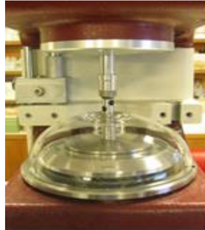
Figure 3.27: the PP25 Ti96010 sensor isolated by a solvent trap in order to limit the water evaporation from the systems.
