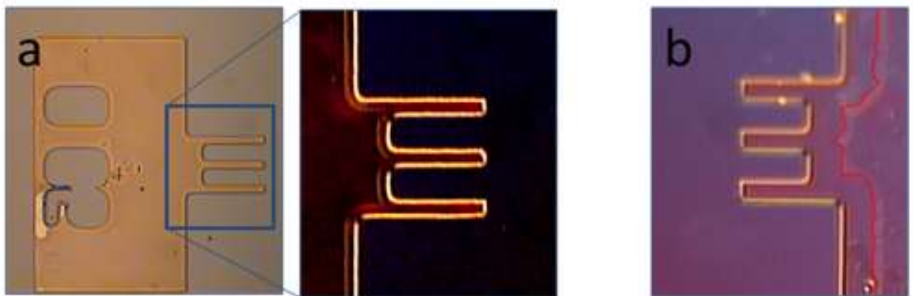
Figure 4.14: a) Before etching silicon oxide layer in HF. b) After HF etching of silicon oxide layer. The dimensions of the cantilevers are changed. The etching profile does not have a symmetric shape under the TCC structure. This can change the mechanical property of the TCC sample.
