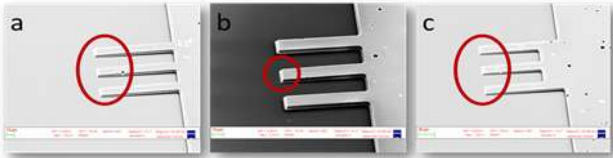
Figure 4.12: These cantilevers are made in silicon. The red circles are illustrating the sticking area in the cantilevers. The sticking happens only at the free ends of the cantilevers. a) and b) All the cantilevers are suspended to a base. The cantilevers are sticking to the silicon oxide. c) The cantilevers are suspended to an overhang. The sticking of the cantilevers is due to the distance between the cantilevers and the substrate. After rinsing the cantilevers in the water, the sticking appears.
