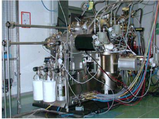
FIGURE 4.4: Photo of the high-mobility MBE system at TASC-IOM-CNR, Trieste
