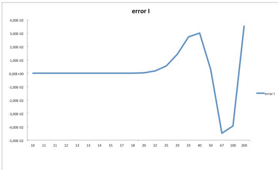
Figure C.20: Relative error in normalized kinetic energy at selected periods between perfect elastic case and the anelastic case.
