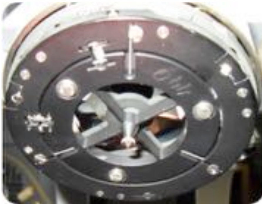
Figure 4: micro-ATR technique, matching a FT-IR microscope with germanium crystal tip (Hyperion 2000, Bruker Optics SpA) with a FT-IR spectrophotometer (Tensor 27, Bruker Optics SpA) and MCT detector
