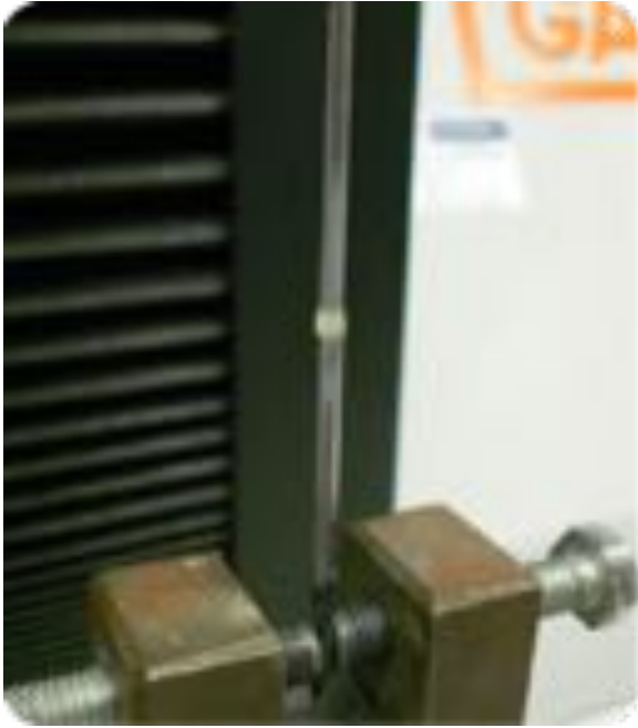
Figure 7: metal rods filled with composite material
