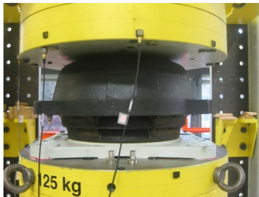
Figure 43 - Resilient mount under test
