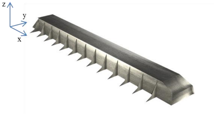
Figure 81 - Half foundation (FE model level 0)
