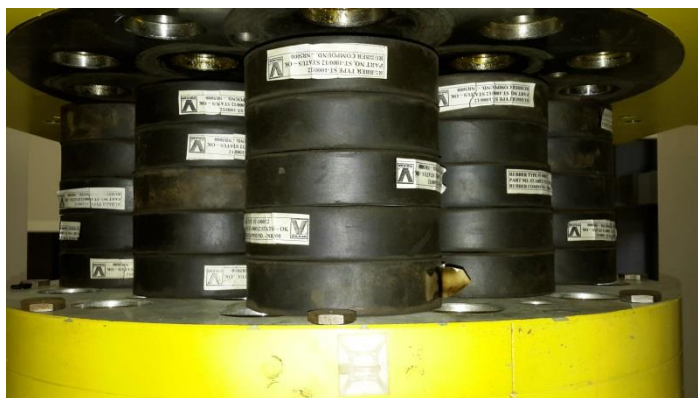
Figure 38 - Rubber disks used as soft isolators
