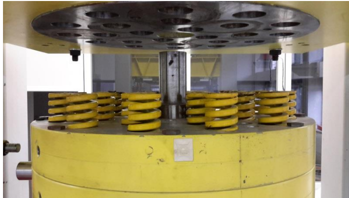
Figure 37 – Steel springs used as soft isolators to decouple the moving system by the rigid frame of the test rig
