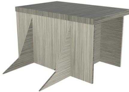
Figure 12 - Typical example of a cell element, part of the diesel engine foundation
