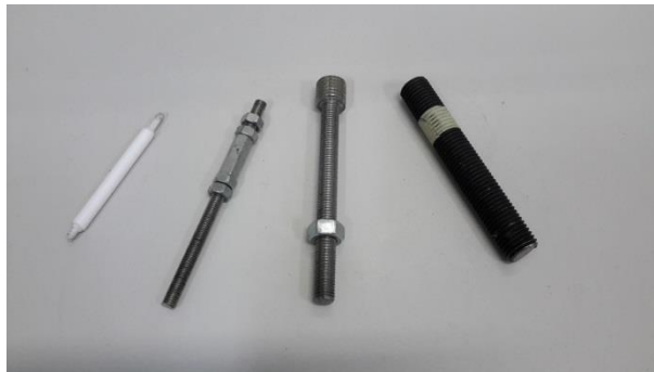
Figure 20 – Different types of stinger rods: (from left to right) nylon rod, M8 steel rod, M12 steel rod, M20 steel rod
