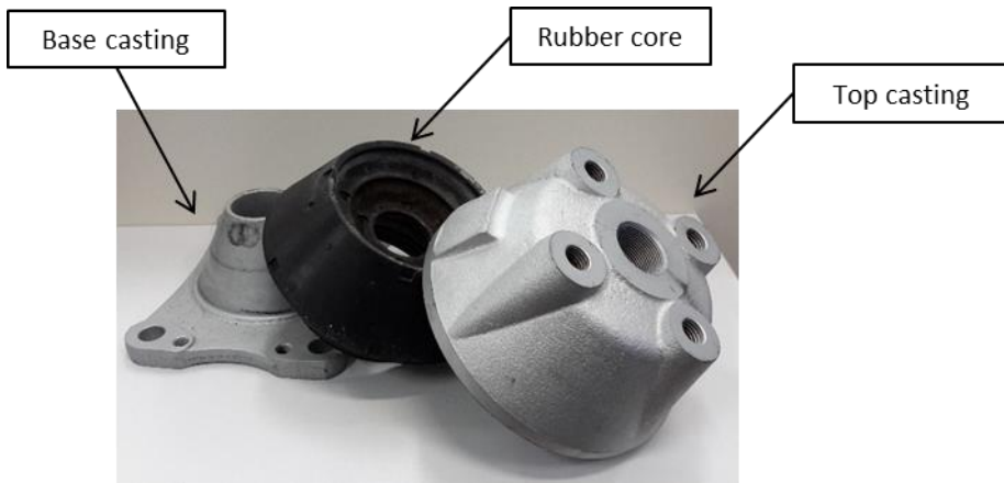
Figure 51- Components of conical passive resilient mount for marine diesel engine
