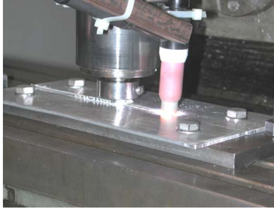
Figure 5.36 – HFSW test were conducted using this simple equipment, in order to demonstrate the working principle on an AA6060-T5 planar sample.
