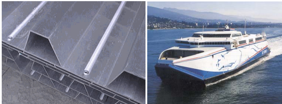
Figure 5.34 – HFSW is well-suited for the fast, highly automatized welding process of thin structures, like that employed for building modern high performances ships.
