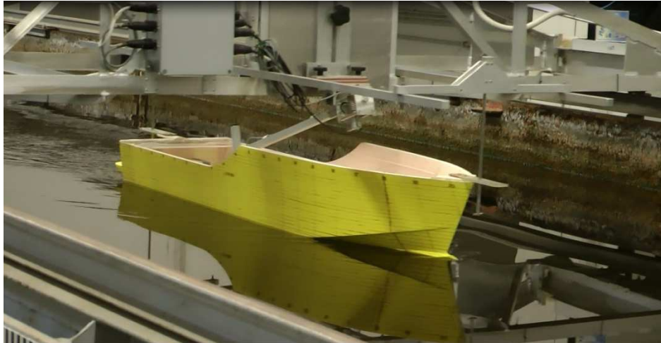
Fig. 7.4 - Tank test of HPH24 at Fr 0.2
