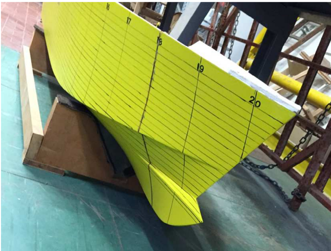
Fig. 7.3 - HPH24 scale model with waterlines and sections
