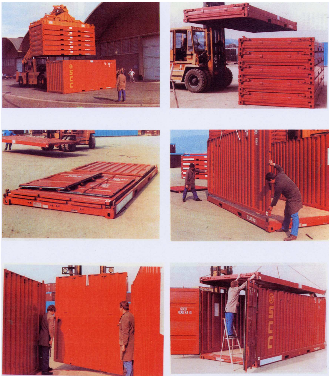
Fig. 2. The folding process of the Six-in-One container Source: SCC Six-In-One containers company S.A.
