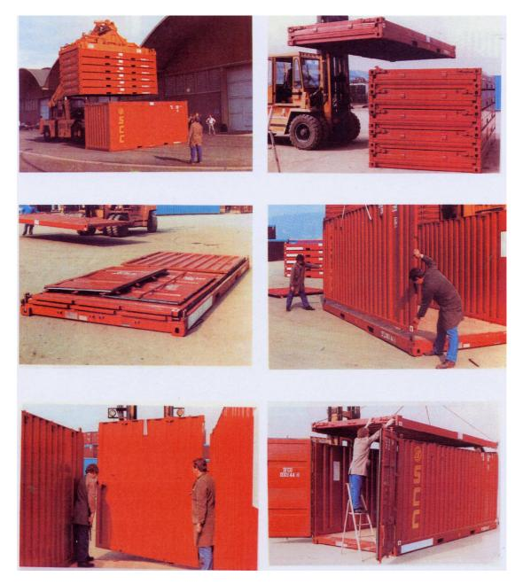
Fig. 2. The folding process of the Six-in-One container Source: SCC Six-In-One containers company S.A.
