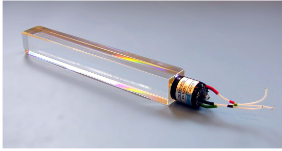
Figure 3.2.6: An example of a \text{PbWO}_4 crystal composing the ECAL calorimeter.
