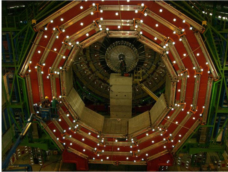
Figure 3.2.10: Picture of the muon chambers embedded in the iron return yoke of the CMS magnet.
