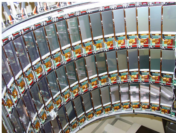
Figure 3.2.5: Layer 5 section of the silicon microstrips detector in the inner barrel region.
