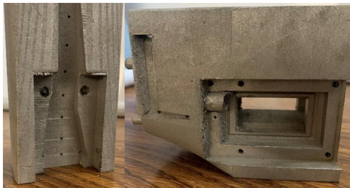
Figure 39: Leading (left), Trailing (right) section of the main body of the model with supports removed.
