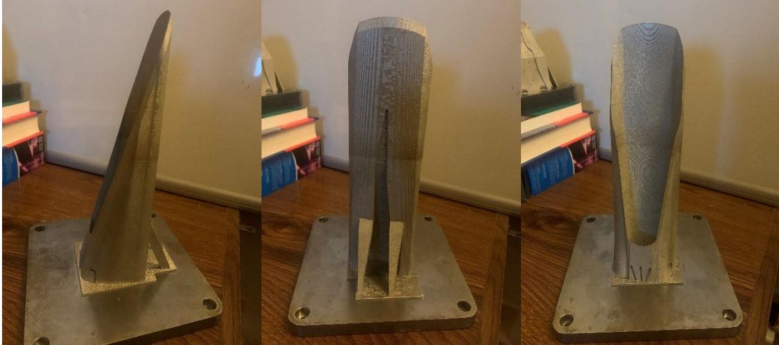
Figure 36: Side (left), Top (center), Bottom (right) views of completed leading section of the model. Note supports from recessed plate edge, Discoloration line due to oxidation, and surface roughness of near vertical edge on body side(top)
