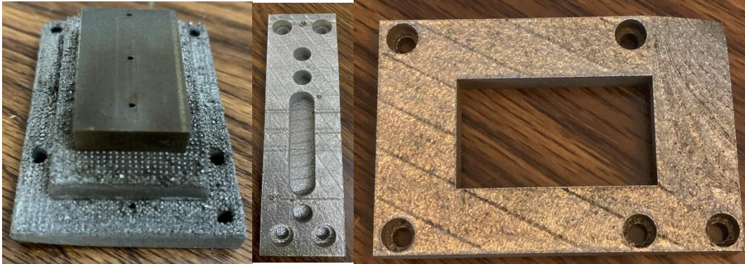
Figure 40: post-processed (left) window blank, (center) recessed plate, (right) window frame.
