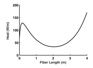
Figure 26: Sample fiber quantum defect profile [reprinted from Yu et al.<sup>20</sup>, Fig. 1]
