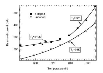
Figure 108: Characteristic temperature T $_0$  for P-doped and undoped quantum dot lasers emitting in the 1.55  $\mu$ m regime<sup>59</sup>
