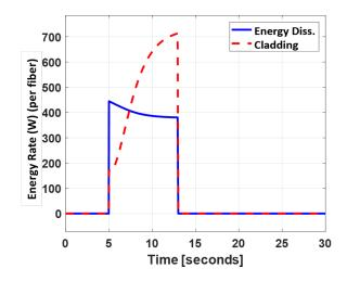
Figure 20: Heat generation in a single active fiber
