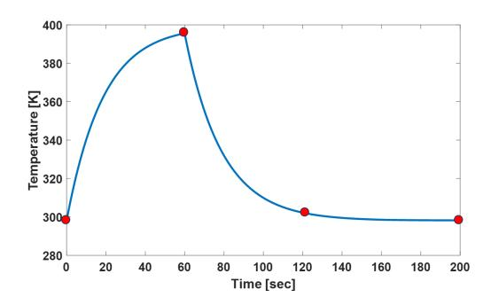
Figure 43: Max fiber temperature with forced convection, velocity of 3 m/s
