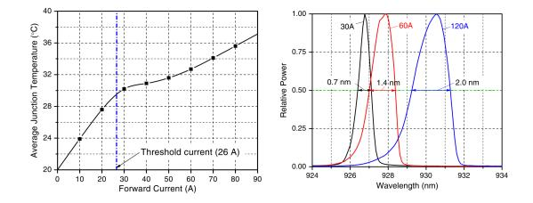
Figure 117: Results showing average junction temperature as a function of forward current and the wavelength shift/spectral broadening due to higher junction temperatures from increased
