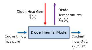
Figure 29: Diagram of laser thermal model
