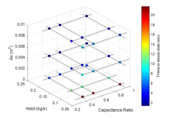
Figure 56: Parameter sweep for time to steady state of T<sub>f</sub> values
