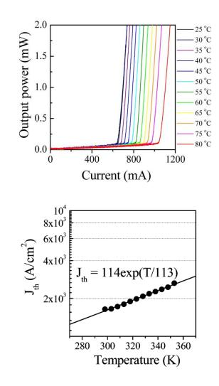
Figure 104: Temperature dependence of L-I characteristic curves and relationship between threshold current density and operating temperature with  $T_0 = 113K^{55}$
