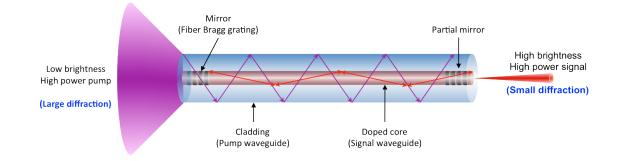
Figure 127: Pump power is converted to signal power through an optical fiber by doping ions in the core, turns large NA pump light into small NA signal light<sup>74</sup>
