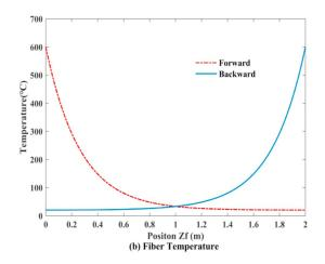
Figure 47: Forward and backward fiber temperature profile [reprinted from Lv et al.<sup>35</sup>, Fig. 5b]
