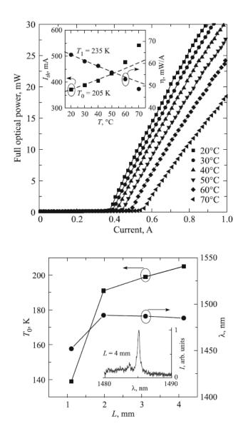
Figure 113: L-I curve at various operating temperatures, both characteristic temperature graphs, and  $T_0$  variation with cavity length  $L^{63}$
