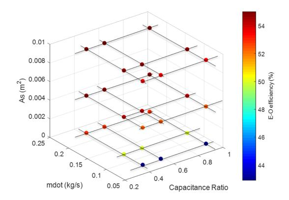
Figure 59: Parameter sweep for overall E-O efficiency of diode array
