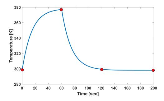
Figure 44: Max fiber temperature with forced convection, velocity of 5 m/s
