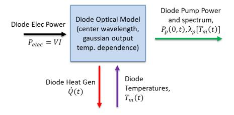
Figure 5: Diagram of laser optical model
