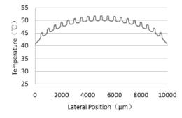
Figure 123: Transverse temperature profile of quantum wells at steady state<sup>72</sup>
