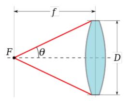
Figure 126: Illustration of relationship between focal length (f) and aperture diameter of lens (D), where F is the focal point (reprinted from Figure 2.4 in Motes et al. <sup>32</sup>).
