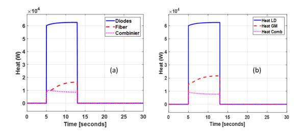
Figure 19: Heat output of rate equation fiber model (a) and simplified model from (b)
