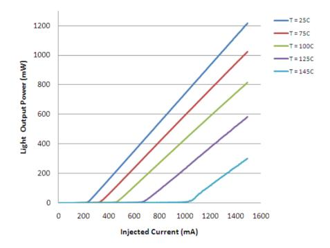
Figure 102: Experimental research showing the trend of increasing threshold current and decreasing slope efficiency due to increasing junction temperature (mW of optical power)<sup>50</sup>
