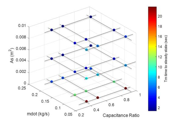
Figure 55: Parameter sweep for time to steady state of  $T_m$  values
