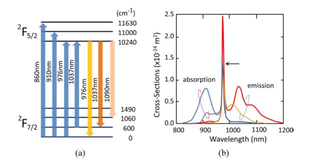
Figure 128: Typical energy level diagram of Yb<sup>3+</sup> ions in silica glass (a) and typical emission and absorption cross-sections in aluminosilicate (thicker lines) and phosphosilicate (thinner lines) fibers. The arrow represents the peak of the phosphosilicate emission/absorption<sup>78</sup>
