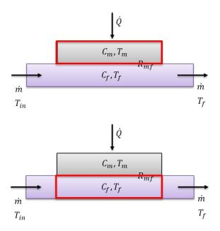
Figure 31: Diagram of control volumes for thermal model analysis
