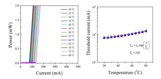
Figure 105: Temperature dependence of L-I characteristic curves and relationship between threshold current and operating temperature with  $T_0 = 102K^{56}$
