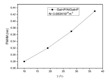
Figure 120: Spectral width changing with heat sink temperature, 0.28, 0.32, 0.37, and 0.43 nm for 10, 19, 28, and 37 °C, respectively<sup>64</sup>. If FWHM is represented by  $\beta$ , then the slope of the line
