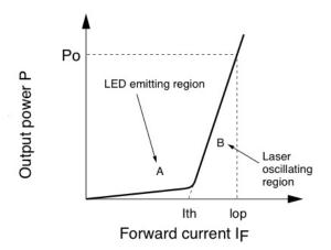
Figure 98: Laser diode threshold current diagram<sup>48</sup>
