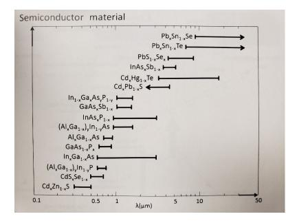
Figure 95: Lasing wavelength for certain semiconductor materials in the active region<sup>46</sup>
