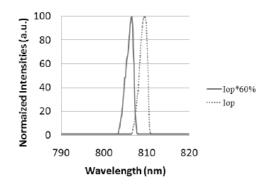
Figure 124: Wavelength of steady state laser bar output for a particular operating current value and 60% of that value<sup>72</sup>
