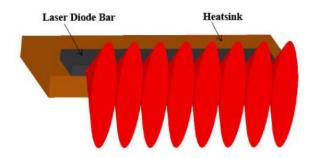
Figure 121: Packaging of a high power semicinductor laser array showing laser output ("fast" divergence axis in vertical direction and "slow" divergence axis in the horizontal direction)<sup>71</sup>
