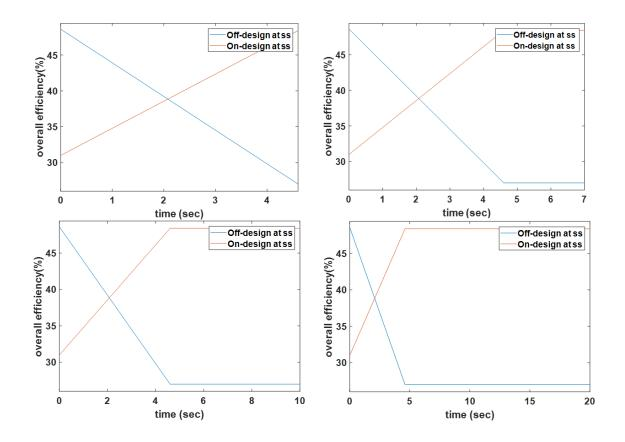
Figure 72: Efficiency plots at varying pulse lengths for cooling methods A and B (Case 2)
