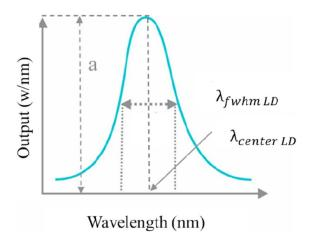
Figure 100: Diagram of Gaussian Curve representing laser diode optical power output<sup>37</sup>
