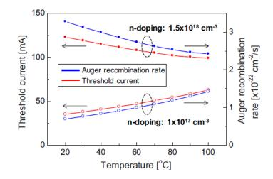
Figure 115: Threshold current vs. operating temperature for 2 n-doping levels<sup>65</sup>
