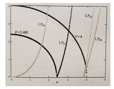
Figure 129: Graphical solution showing V cutoff points for various LP modes. Parameters w and u come the planar waveguide mode derivation of Maxwell's equations and are defined such that
