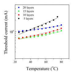
Figure 106: Relationship between threshold current and operating temperature with a varying number of quantum dot layers. The  $T_0$  values for each sample were 51K for N = 5, 91K for N = 10,
