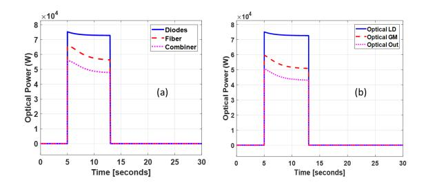
Figure 18: Optical power output of rate equation fiber model (a) and simplified model (b)
