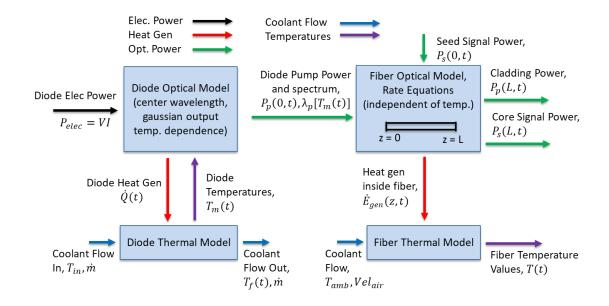
Figure 4: Diagram of all coupled models for entire laser system
