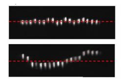
Figure 122: Laser bar "smile" showing a good spectrum vs. a bad spectrum<sup>71</sup>. A laser bar is operating optimally when the spectrums of all emitters are the same<sup>71</sup>
