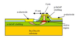
Figure 96: Typical laser diode diagram showing materials/components for operation<sup>47</sup>
