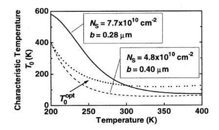
Figure 116: Experimental results of characteristic temperature  $T_0$  as a function of laser diode operating temperature<sup>53</sup>
