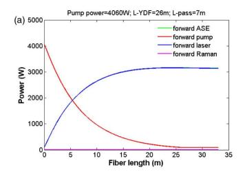
Figure 24: Pump and signal power levels [reprinted from Yu et al.<sup>100</sup>, Fig. 7a]
