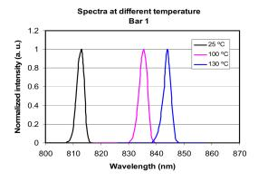
Figure 118: Wavelength shift due to higher junction temperatures from increased forward current in an 808 nm laser diode<sup>67</sup>
