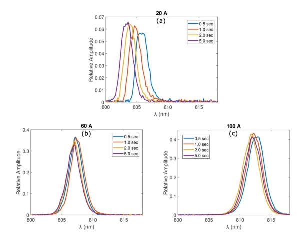
Figure 13: Golden Bullet spectrum output at various current levels<sup>70</sup>
