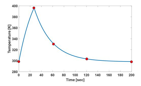
Figure 42: Max fiber temperature with forced convection, velocity of 1 m/s
