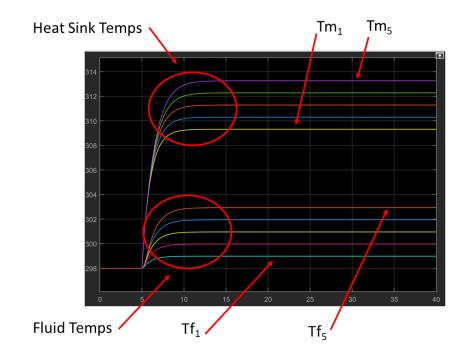
Figure 50: Thermal model data explanation
