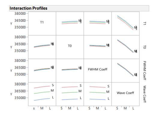
Figure 64: Interaction profiles for wavelength coefficient ( $d\lambda/dT$ ), FWHM coeffcient ( $d\beta/dT$ ),  $T_0$ and  $T_1$ , showing the effects of each parameter on optical energy out<sup>38</sup>
