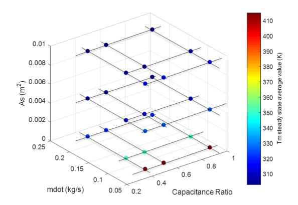
Figure 51: Parameter sweep for average T<sub>m</sub> steady state values
