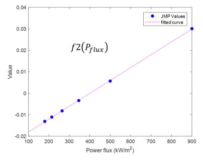
Figure 79: Data plot for f2 curve of  $T_m^*$  equation
