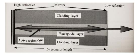
Figure 97: Explanation of laser diode operation using the Fabry-Perot Resonator<sup>46</sup>
