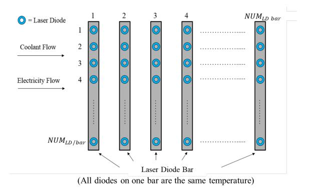
Figure 6: Laser diode array diagram<sup>37</sup>
