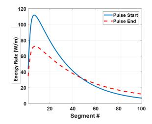
Figure 23: Fiber heat deposition profiles at beginning (t = 5 sec) and end (t = 13 sec) of activation
