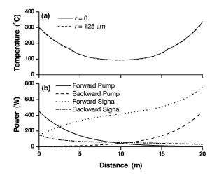
Figure 49: Fiber temperature profile [reprinted from Wang et al.<sup>13</sup>, Fig. 2]
