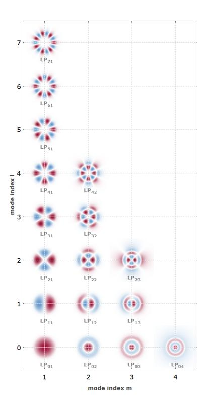
Figure 130: Generic intensity profiles for guided  $LP_{l,m}$  modes of a fiber with V =11.4. The two colors indicate positive (red) and negative (blue) signs of the electric field<sup>79</sup>
