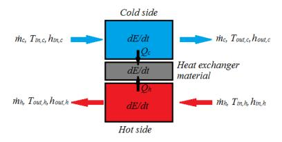
Figure 33: Diagram of heat exchanger thermodynamic model<sup>98</sup>
