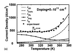
Figure 109: Graph showing invariant threshold current ( $T_0 = \infty$ ) in the range of 278 to 348K<sup>60</sup>
