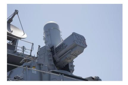
Figure 2: Helios LWS delpoyed on a navy ship<sup>9</sup>
