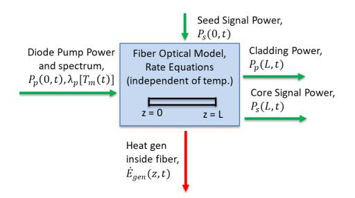
Figure 8: Diagram of fiber optical model
