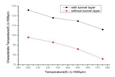
Figure 111: Laser characteristic temperature  $T_0$  as a function of junction temperature comparing the performance of an InGaAsP laser diode with and without a tunnel barrier<sup>61</sup>
