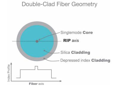
Figure 125: Diagram of fiber geometry with core, inner cladding, and outer cladding. The refractive index profile (RIP) of each layer is given to show how its magnitude changes<sup>73</sup>
