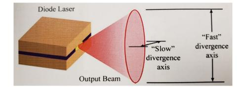
Figure 99: Diagram Denoting the "Fast" and "Slow" Axis of Laser Diode Output<sup>46</sup>
