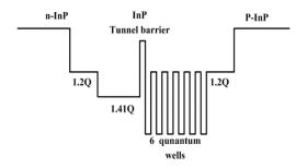
Figure 110: Schematic of InGaAsP/InP MQW laser with tunnel layer<sup>61</sup>
