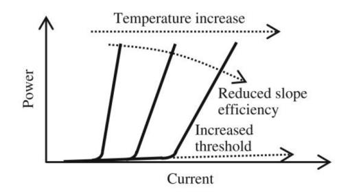
Figure 101: Generalized graph of optical output power vs. forward current showing the effects of junction temperature on threshold current and slope efficiency<sup>49</sup>
