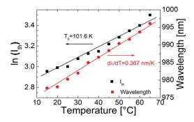
Figure 107: Operating temperature versus the natural log of threshold current and lasing wavelength showing  $T_0 = to 101K$  and wavelength temperature coefficient  $d\lambda/dT = 0.367 \text{ nm/K}^{58}$ The  $T_0$  value found by Arsenijević et al. can be confirmed using equation 77 and estimations from the figure above as shown here.
