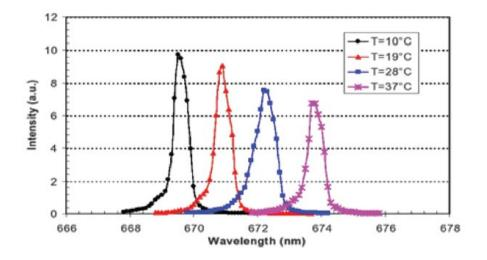
Figure 119: Laser diode output intensity changing with wavelength shift due to shifting heat sink temperature<sup>64</sup>
