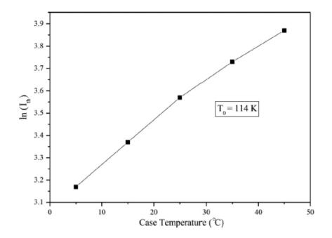
Figure 114: Threshold current vs. operating temperature, slope of curve is  $T_0 = 114K^{64}$
