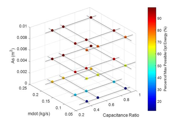
Figure 62: Parameter sweep for percent of maximum possible optical energy
