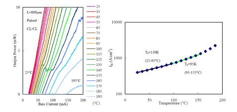
Figure 112: L-I curves at various operating temperatures and operating temperature vs. threshold current density plots<sup>62</sup>
