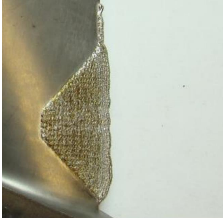
Figure 25: Final product of an LBP-DED repair deposit on an IBR blade before being polished back to nominal geometry
