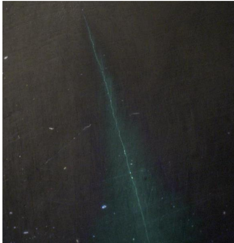
Figure 6: Crack found using FPI on a vibration fatigue specimen
