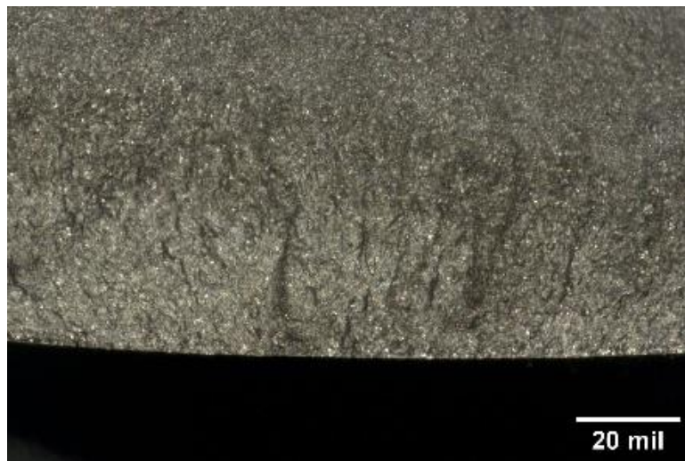
Figure 32: Initiation point on the fracture surface of blade a.) A-3, b.) B-4, and c.) C-5.
