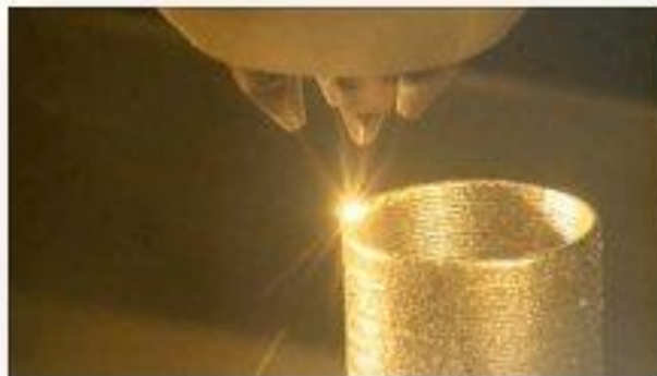
Figure 4: Directed energy deposition using blown powder as the feed source for the metal alloy. [11]
