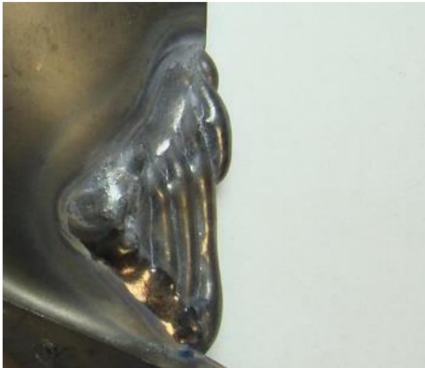
Figure 18: Final result of a wire DED process repair deposit before it was polished back to nominal geometry
