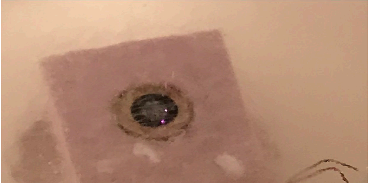
Figure 4-3. Image of the YBCO ring while in the LN2 bath with the laser incident.
