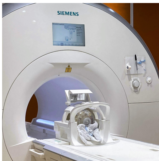
Figure 4.1: Diffusion phantom in its axial orientation within a head/neck coil. A 3D-printed base holder and stabilizing aids were used to assist in reproducible positioning
