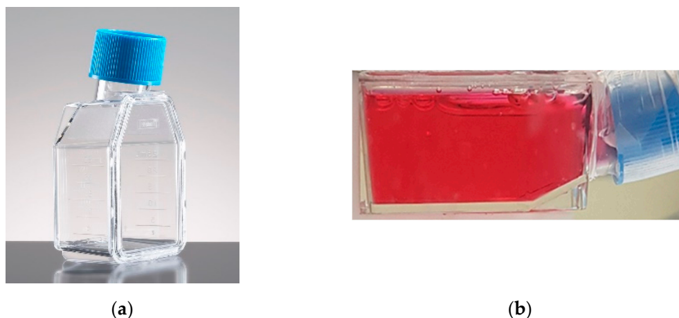
Figure 7. (a) A 12.5 cm 2 culture flask, as the ones used; (b) the same flask containing the cell layer and the culture medium, ready for irradiation.
