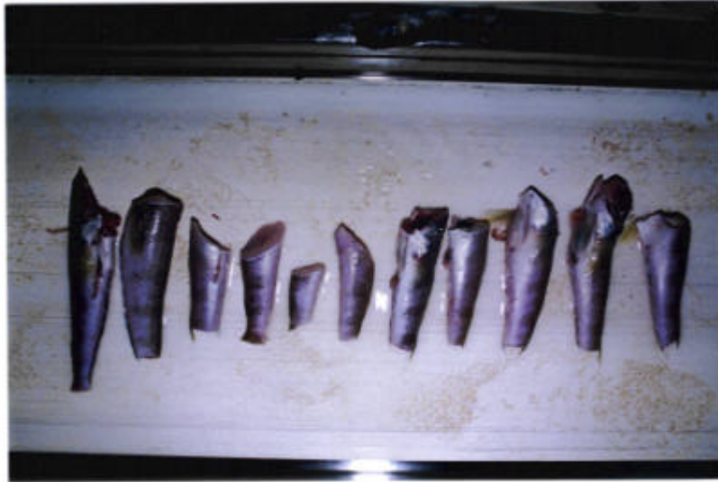
Fig. 8. BAADER 424 Cont. Uneven output of the BAADER 424.
