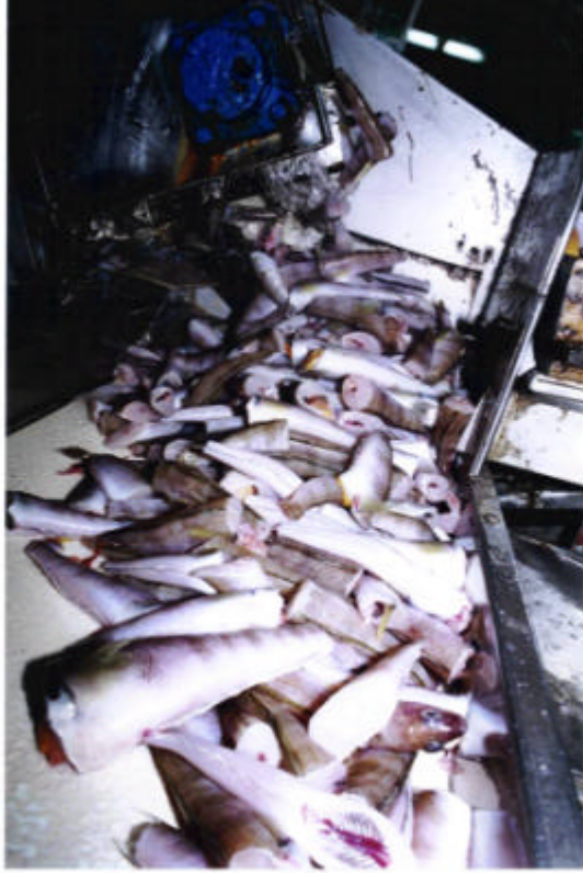
Fig. 10. P. Ramsayi trunks (headed, tailless and gutted) going out from the washing machine and ready to be packed.
