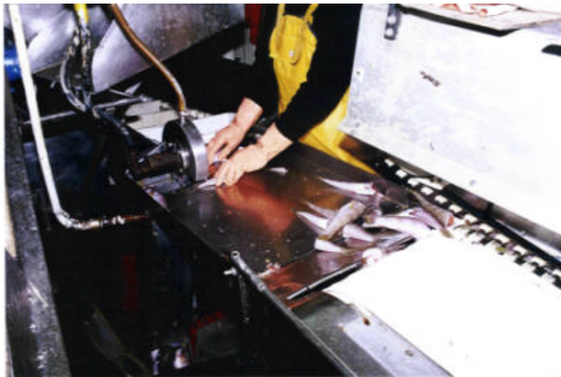
Fig. 9. Once headed the fish pass through a “tail cutter” and then to a gutting basin before to go into the washing machine.
