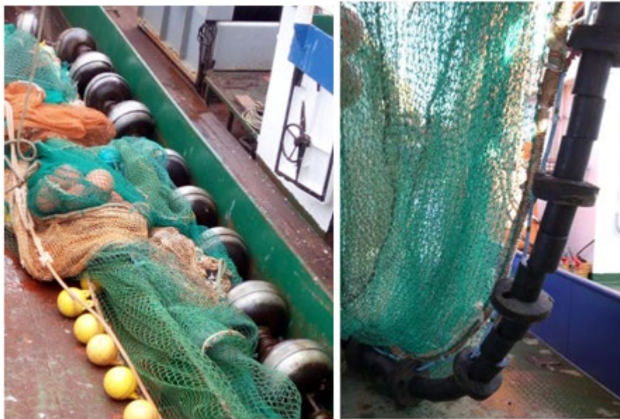
Figure A.5.15.2 - NCT footrope: Left with rollers, Right with new rubber disks
