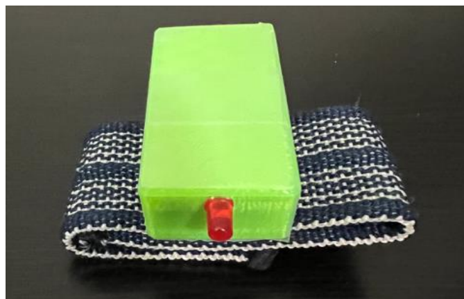
Fig. 2. The Staff Module can be worn on one's wrist or bicep. The prototype is shown with a custom 3D-printed enclosure.
