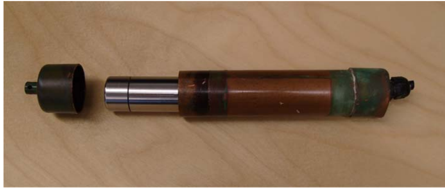
Figure 2. Underwater transducer protection using a copper jacket
