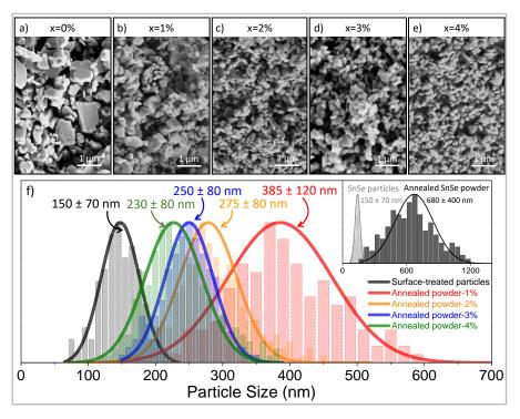
**Figure S4.** Representative SEM images of annealed nanopowders: a) SnSe, b) SnSe-1%CdSe, c) SnSe-2%CdSe, d) SnSe-3%CdSe and e) SnSe-4%CdSe. f) The particle size distributions histograms and corresponding average size obtain by measuring more than 100 particles.
