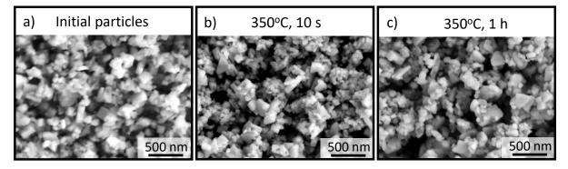
**Figure S9.** Representative SEM images of a) initial SnSe paticles; b) annealed SnSe nanopowder at 350°C for 10 s; c) annealed SnSe nanopowder at 350°C for 1 h. It can be seen there is only little difference in the grain size of bare SnSe annealed up to 350°C.
