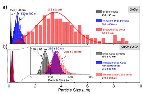
Grain size evolution study for bare SnSe and SnSe-3%CdSe
