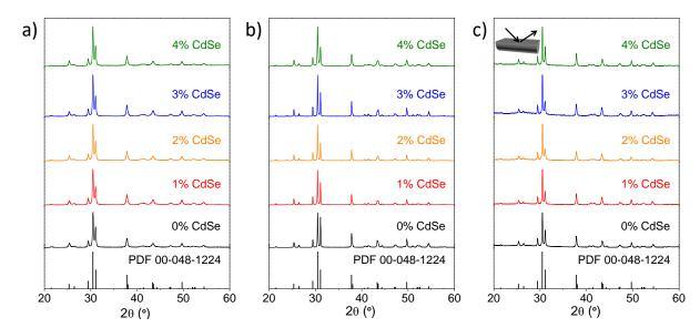
XRD patterns of SnSe and SnSe-x%CdSe nanocomposites
