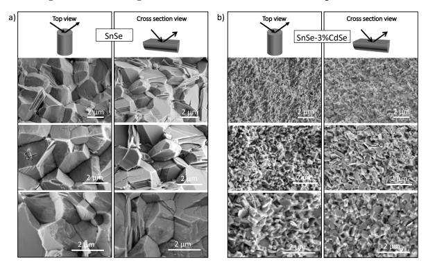
SEM images at different magnifications of SnSe and SnSe-3%CdSe pellets
