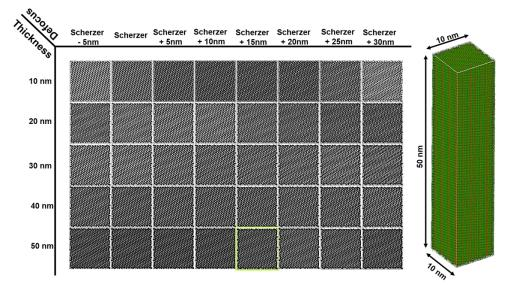
**Figure S25.** SnSe *Pnma* image simulation as a function of crystal model thickness and defocus condition. The initial 3D atomic model is  $10 \text{ nm} \times 10 \text{ nm} \times 50 \text{ nm}$  big to reproduce the image contrast reported in Figure 24e. Later the thickness has been reduced with 10 nm steps to investigate thickness related main features.
