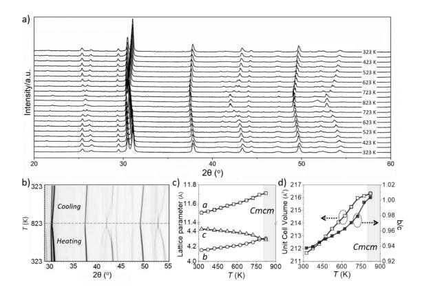
**Figure S15.** High-temperature XRD analyses of SnSe-3%CdSe nanocomposites: a) the evoluation of XRD patterns with the change in temperature from 323 to 823 K followed by subsequent cooling to 323 K; b) 2D plot of intensity as a function of  $2\theta$  and T; c) the lattice parameters, and d) lattice parameter ratio b/c and unit cell volume as a function of temperature.
