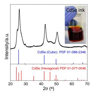
**Figure S8.** XRD pattern of recrystallized CdSe upon annealing at 350 °C, the inset shows the initial molecular complexes solution of CdSe in the en-EDT mixture including reference
