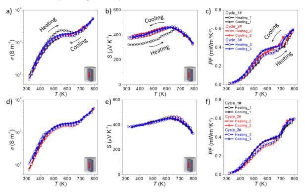
**Figure S26.** The temperature dependence of (a, d) electrical conductivity ( $\sigma$ ), (b, e) Seebeck coefficient (*S*) and (c, f) power factor (*PF*) of a SnSe-3%CdSe pellet. a)-c) No pre-stabilization treatment was carried out before the measurements; d)-f) Pellet was annealed in forming gas atmosphere before the measurements. For details, please refer to the section "*bulk nanomaterial consolidation*" in the main text.
