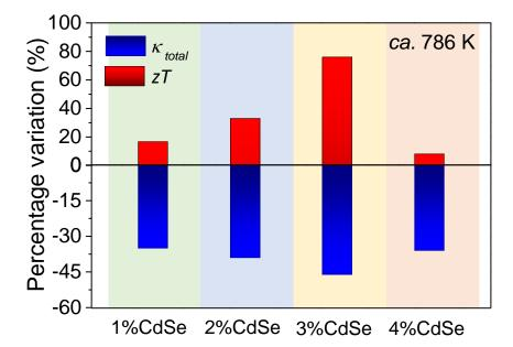
Percentage variations in the TE properties of SnSe-x%CdSe compared to SnSe
