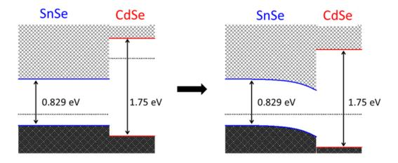
**Figure S19.** Representation of the band structure changes in SnSe induced by the CdSe NPs in the SnSe/CdSe interface.
