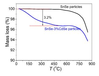
Figure S12. TGA of the original SnSe particles, and SnSe-3%CdSe particles.
