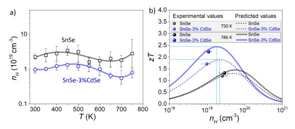
**Figure S29.** a) Temperature dependence of the Hall charger carrier concentration,  $n_H$ ; b)  $n_H$ dependent zT with both experimental and predicted values at T=750 K and 786 K *via*calculations using the SPB model. The light blue dashed lines indicate the optimal carrier
