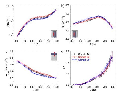
**Figure S27.** Thermoelectric properties of three SnSe-3%CdSe pellets obtained three different batches: a) electrical conductivity,  $\sigma$ ; b) Seebeck coefficient, *S*; c) thermal conductivity,  $\kappa_{total}$ ; and d) figure of merit, *zT*.
