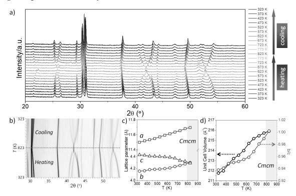
High-temperature XRD analyses of SnSe and SnSe-3%CdSe
