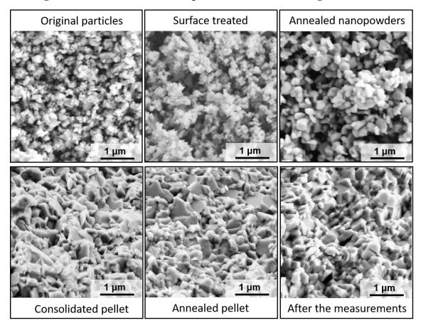
SEM images of SnSe-3%CdSe nanocomposites at the different stages
