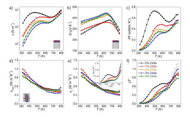
**Figure S18.** TE properties of bare SnSe and SnSe-x%CdSe (x = 0, 1, 2, 3, and 4) samples measured in perpendicular to the pressing direction: a) electrical conductivity,  $\sigma$ ; b) Seebeck coefficient, *S*; c) power factor, *PF*; d) thermal conductivity,  $\kappa_{total}$ ; e) lattice thermal conductivity,  $\kappa_L$ , electronic thermal conductivity,  $\kappa_e$  (inset); and f) figure-of-merit, *zT*.
