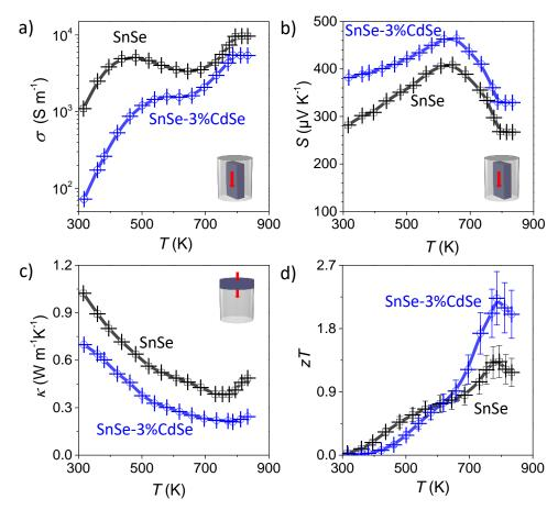
TE properties of SnSe and SnSe-3%CdSe measured in parallel direction
