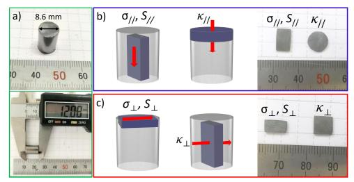
**Figure S28.** a) Photograph of a cylindrical pellet produced by spark plasma sintering (SPS). (b, c) Schematic illustrations and photographs of the samples obtained from the cylindrical pellets and used to measure TE properties in each direction: parallel b) and perpendicular c) to
