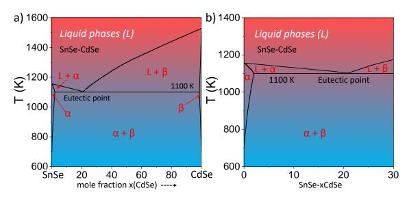
**Figure S13.** a) Complete SnSe-CdSe phase diagram and b) magnification of the low CdSe content region.<sup>1</sup>
