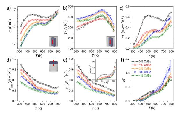
TE properties of SnSe-CdSe samples with different content of CdSe
