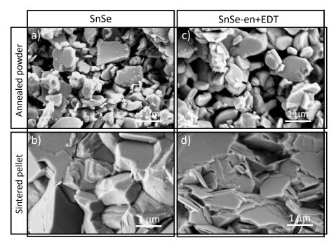
**Figure S11.** Representative SEM images of the a) annealed SnSe particles, b) corresponding cross-section of sintered SnSe pellet; c) annealed SnSe previously treated with the en+EDT mixture, and d) the corresponding cross-section of the sintered pellet.
