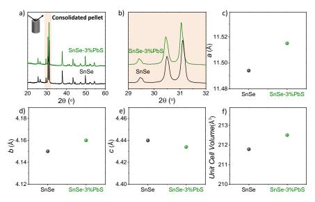
**Figure S16.** a) XRD patterns of bare SnSe and SnSe-3%PbS pellets in the perpendicular to the pressing axis; b) Magnification of the XRD pattern for the consolidated pellets with and
