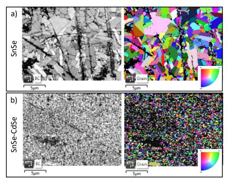
**Figure S7.** EBSD microstructure of a) bare SnSe and b) SnSe-3%CdSe nanocomposite pellet. On the left of a) and b): the band contrast images of bare SnSe and SnSe-3%CdSe nanocomposite pellet, respectively. On the right of a) and b): the grain color images of bare SnSe and SnSe-3%CdSe nanocomposites, respectively.
