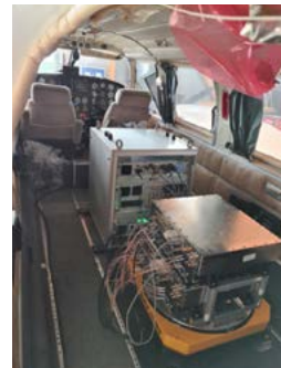
Figure 1. OSCAR system inside the aircraft, showing the mounted gimbal, radio-frequency unit and analog-to-digital converter on the bottom right.
