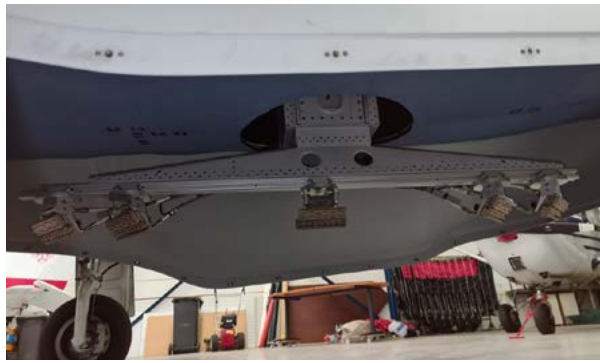
Figure 2. OSCAR system mounted on the belly of the aircraft. The mounted antenna frame shows one single broadside antenna in the middle and two squinted antennas pairs on either side looking 45° fore and aft of the broadside direction.
