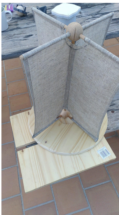
Figure 14. One of the experimental drifters made with wood and linen canvas.
