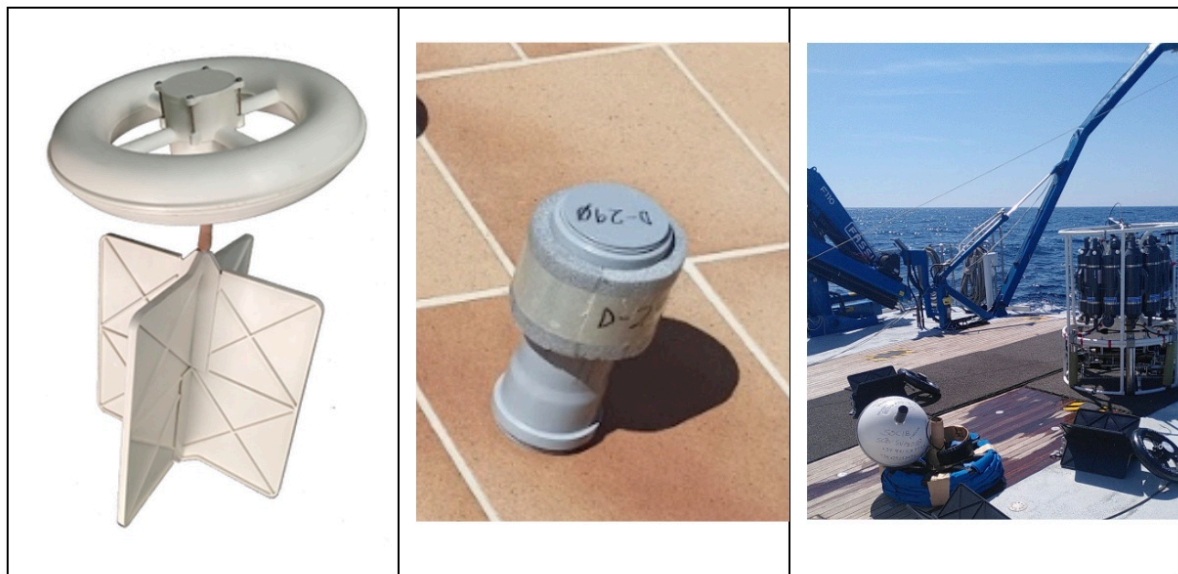
Figure 13. Surface drifters to be deployed. Left: CARTHE drifter (source: https://www.pacificgyre.com/carthe-drifter.aspx ). Middle: HEREON drifter. Right: SVP-B drifter.
