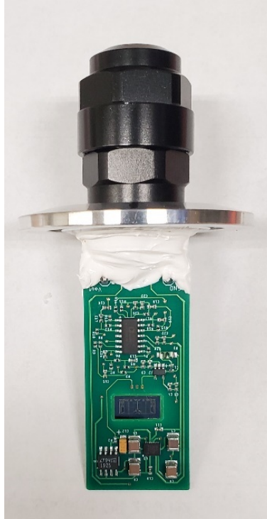
Figure 36. Gen 6 sensor assembly modified with marine sealant.
