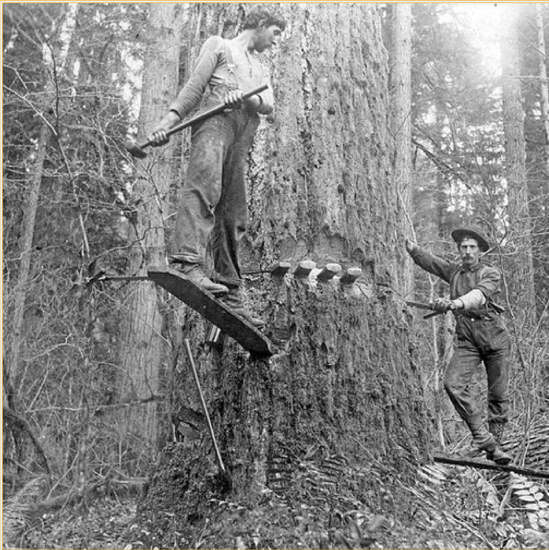
Two loggers with springboards pounding wedges into tree. OSU Special Collections & Archives Research Center Large Wood, Long Legacy
