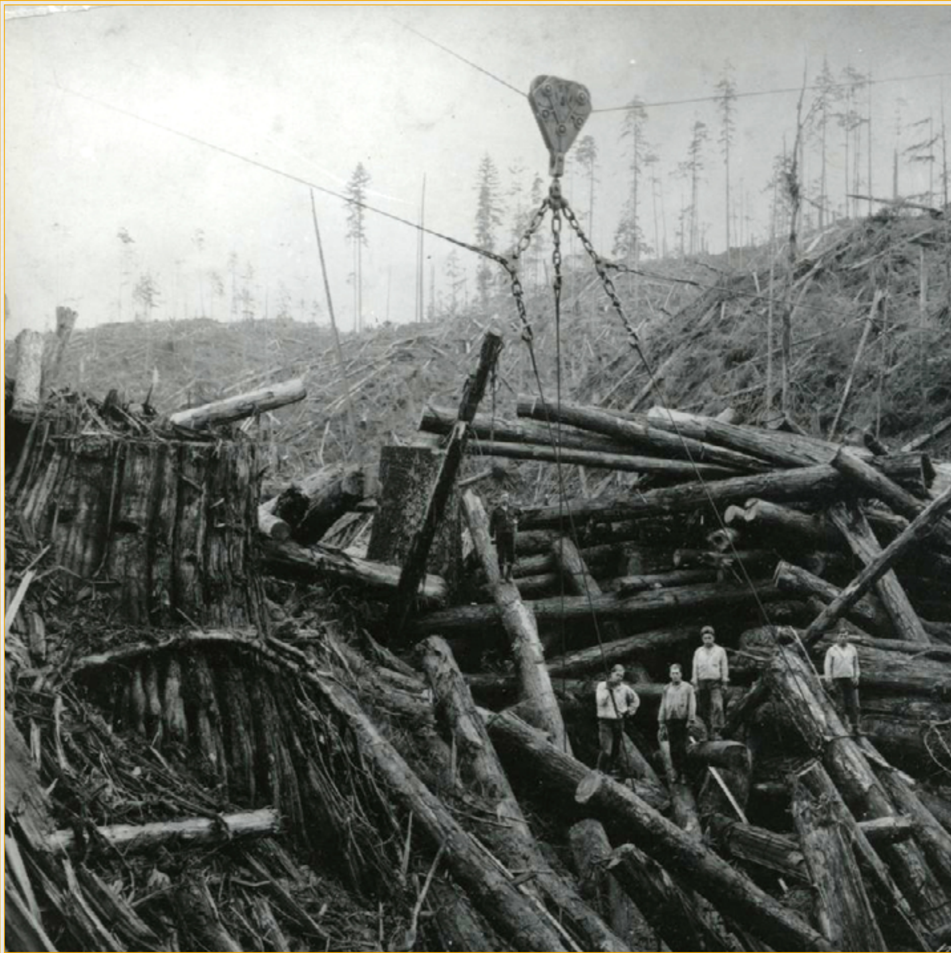
Cold-decking fir, cedar, spruce, and hemlock, Gray's Harbor. Courtesy Oreg. Hist. Soc. Research Lib., 017406 Large Wood, Long Legacy
