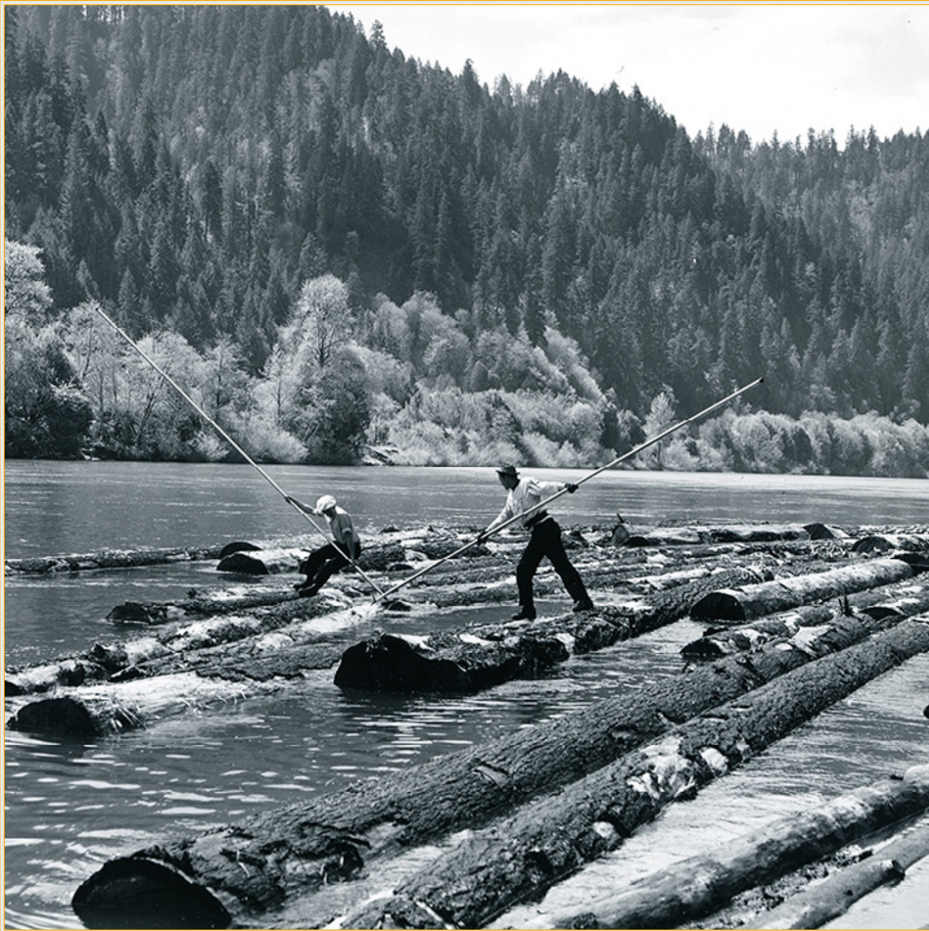
Men use long poles in 1951 to maneuver logs into rafts to float on the Umpqua River to a mill for processing. (Oregon State Archives)
