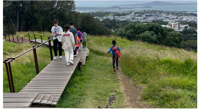
Figure 96: Limitation of boardwalk width leads to alternative paths and 'desire line' scarring. Author's own image.
