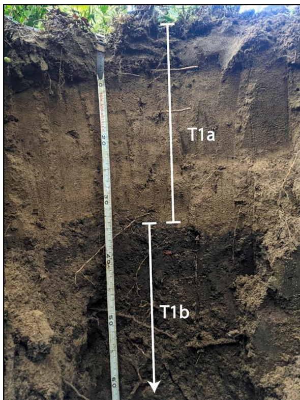
Fig. A1. Annotated photo of Terrace 1. T1a (top) is light in color, coarse, sandy, and relatively unweathered material. T1b is the first buried soil and is much darker in color and composed of finer grained matrix.
