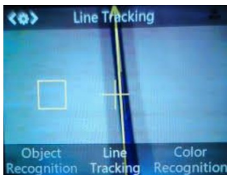
Figure 6. Line tracking with huskylens camera
