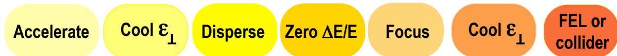
FIGURE 1. Stages of Laser-Plasma Staged FEL: acceleration, cooling transverse degrees of freedom, dispersing the beam, monochromatization, focusing, one more transverse cooling stage, and sending the cooled beam to an FEL undulator or, for use in a collider.
