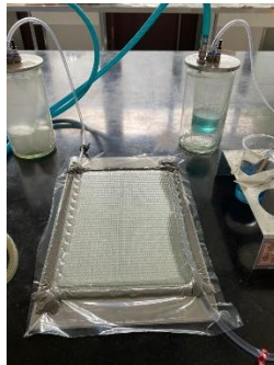
Fig. 1: A typical VARI infusion process set-up for composite manufacturing
