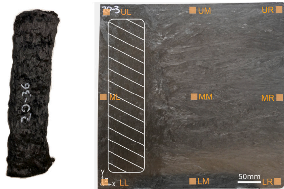
Fig. 4. Left: Photo of a plastificate/initial charge that is inserted in the press. Right: Image of one of the plaques with approximate areas of sample withdrawal in transparent orange and the area of insertion of the plastificate/initial charge in the white patterned area.
