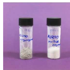
Figure 3. Synthesis and purification of [H 2 B·NMeH] n on 1 g scale.
