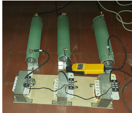
Figure 7. View of the experimental shared three-phase RL load.
