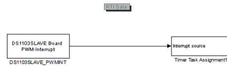
Figure 15. View of the dSPACE's Simulink block DS1103SLAVE_PWMINT connected to the block 'Timer Task Assignment' to make the slave DSP's interruption available.
