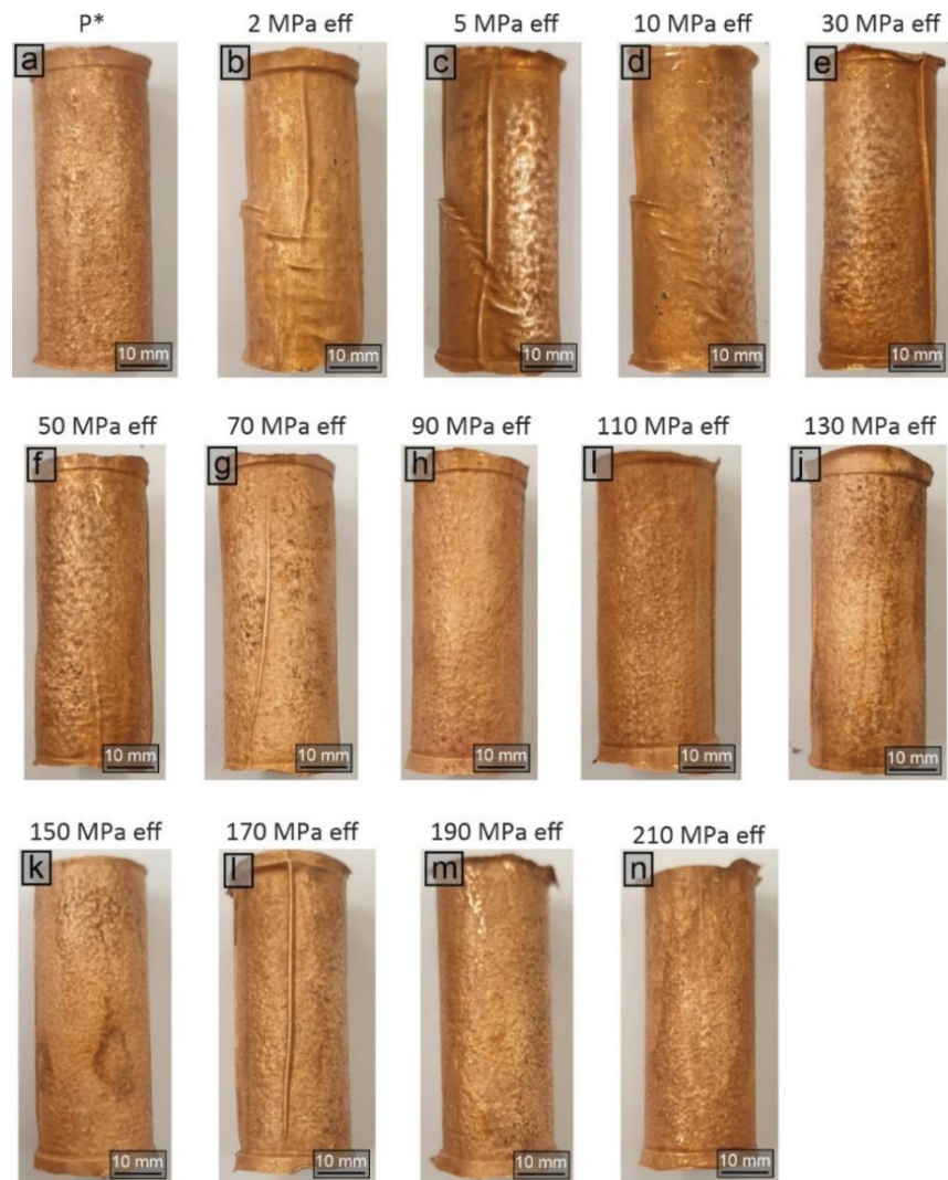
Supplementary Figure 6.1. Castlegate Sandstone samples in their copper jackets, post-deformation. For samples 2–50 MPa, the strain was recorded sufficiently in the jacket to establish the angle at which to cut along their long axes for SEM analysis. For samples 150–210 MPa, the subperpendicular nature of the compaction bands that formed meant that these could be cut lengthways at any position. However, samples 70–130 MPa were analysed using an X-ray micro-CT to identify the orientation of the localised structures in 3D, since these samples showed no significant evidence of strain localisation in the jackets and much of the deformation was assumed to not have formed subperpendicular to \sigma_1 .
