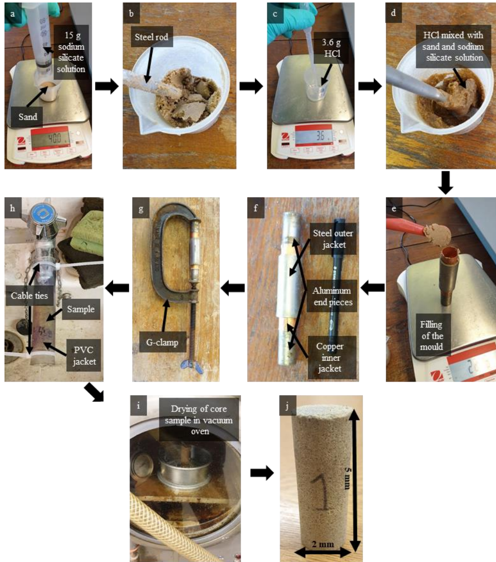
Figure 3.1. Simplified workflow used to create the synthetic sandstone cores. See main text for description of the different steps in the production procedure.
