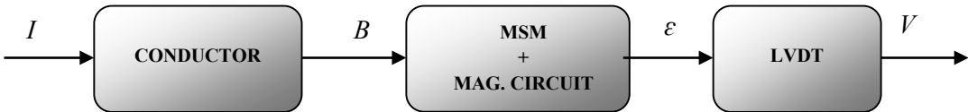
Figure 4.4.2 – Schematic showing the proposed current-measurement system based on (MSM) alloys (with concentrator)
