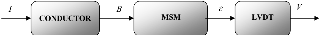
Figure 4.4.1 – Schematic showing the proposed current measurement system based on magnetic shape memory (MSM) alloys [84]
