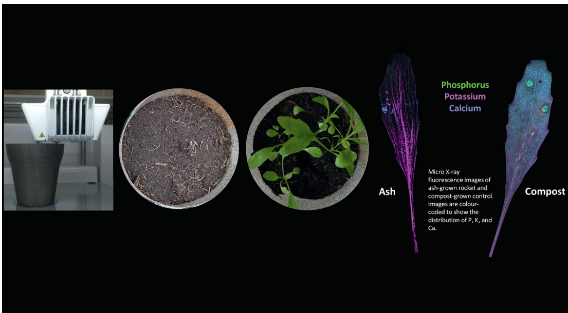
Fig. 4. Experimental set-up for growing plants in La Palma ash—a possible lunar regolith simulant. Left: 3D printing of plant pots using La Palma ash and sustainable PLA bioplastic binder. Second left: Plant pot filled with 75 percent La Palma ash and 25 percent compost; Third left: Rocket growth after 50 days in 75 percent ash; Right: micro-XRF images of leaves from the experiments, with a clear difference seen between the nutrient uptake of the 100 percent compost trial compared with the ash experiment (75 percent ash: 25 percent compost).
