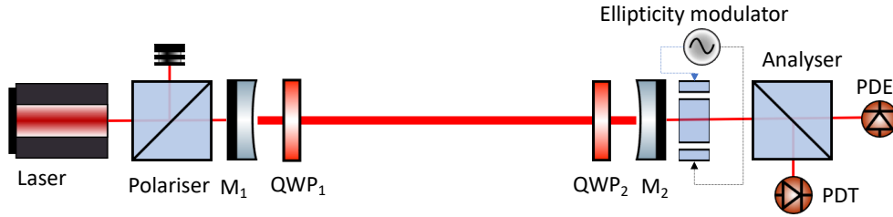
Figure 3.11. The proposed polarimetry experiment for searching for axion-like pseudoscalar fields, which uses a Fabry-Pérot cavity and two quarter-wave plates ( \text{QWP}_1 and \text{QWP}_2 ). PDT, PDE are the photodiodes in the transmission and in the extinction port of the analyser, respectively, and M_1/M_2 are mirrors that delimit the Fabry-Pérot cavity.
