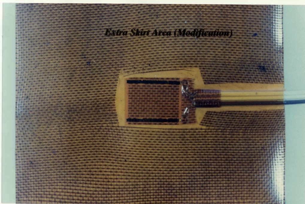
FIGURE 4.3 : MODIFIED RESISTANCE TEMPERATURE DETECTOR (RTD)
