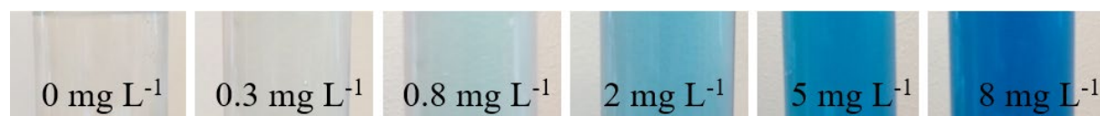
Fig. 1. Photographs of test tubes showing the colour appearance developed 28 min (reaction temperature 21°C) after addition of reagent B for blank (0.1 mol L -1 NaOH), and standard cyanide solutions.
