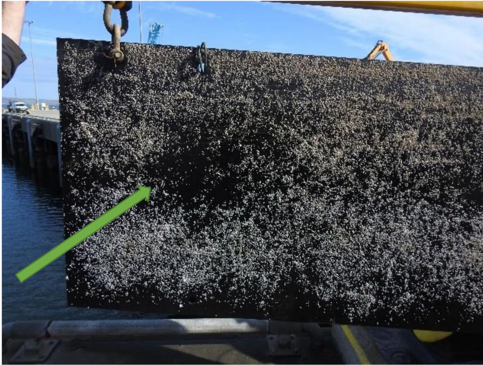
Figure 17. Biofouling removal using an HPUT. The green arrow shows the location of the HPUT at the back of the plate.
